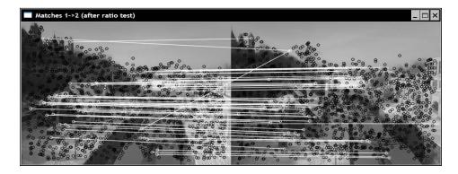
The white lines linking the matched points show that even if we have a large number of good matches, a significant number of false matches have survived. Therefore, a second test will be performed in order to filter our more false matches. Note that the ratio test is also applied to the second match set.
