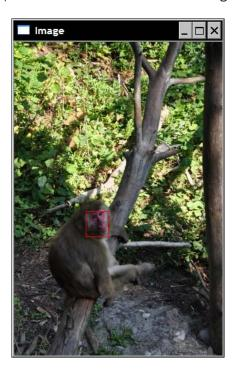
This time, we will describe this object by using the hue channel of the HSV color space. This means we need to convert the image into an HSV one, then extract the hue channel and compute the 1D hue histogram of the defined ROI:
