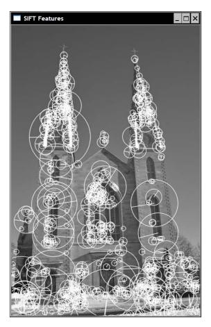
However, since the computation of the feature point is based on floating-point kernels, it is generally considered to be more accurate in terms of feature localization in space and scale. Although, for the same reason, it is also more computationally expensive.
