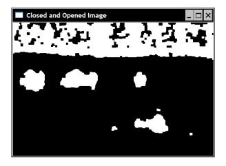
It should be noted that applying the same opening (and similarly the closing) operator on an image several times has no effect. Indeed, with the holes having been filled by the first opening, an additional application of this same filter will not produce any other changes to the image. In mathematical terms, these operators are said to be idempotent.
