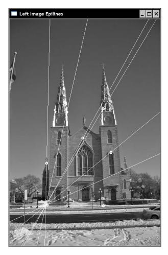
Remember that the epipole is at the intersection point of all epipolar lines, and it is the projection of the other camera center. This epipole is visible on the preceding image. Often, the epipolar lines intersect outside the image boundaries. It is at the location where the first camera would be visible if the two images were taken at the same instant. Observe the image pair and take the time to convince yourself that this indeed makes sense.
