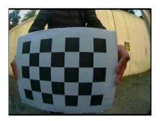
The nice thing is that OpenCV has a function that automatically detects the corners of this chessboard pattern. You simply provide an image and the size of the chessboard used (number of vertical and horizontal inner corner points). The function will return the position of these chessboard corners on the image. If the function fails to find the pattern, then it simply returns false:
