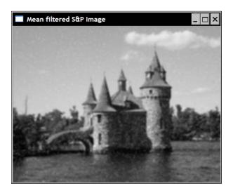
Clearly, the noisy pixels shifted the mean value of neighboring pixels. As a result, the noise is still visible even if it has been blurred by the mean filter.
