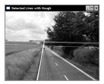
As it can be seen, the Hough transform simply looks for an alignment of edge pixels across the image. This can potentially create some false detection due to an incidental pixel alignment, or multiple detections when several lines pass through the same alignment of pixels.
