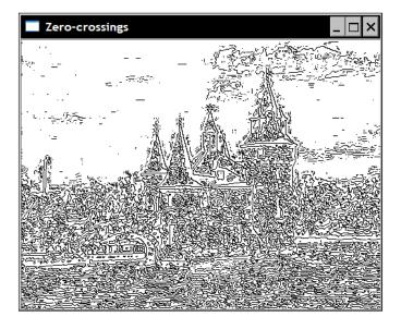
As you can see, the zero-crossings of the Laplacian detect all edges. No distinction is made between strong edges and weaker edges. We also mentioned that the Laplacian is very sensitive to noise. These two facts explain why so many edges are detected by the operator.
