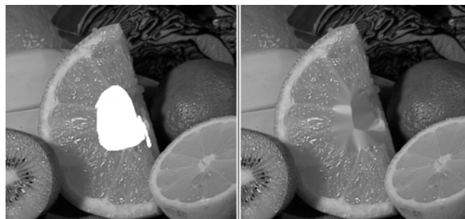
Figure 6-27: Inpainting cannot magically restore textures that are completely removed: the navel of the orange has been completely blotted out (left); inpainting fills it back in with mostly orangelike texture (right)
