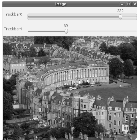
Figure 4-2: A simple application displaying an image; this window has two trackbars attached named "Trackbar0" and "Trackbar1"
