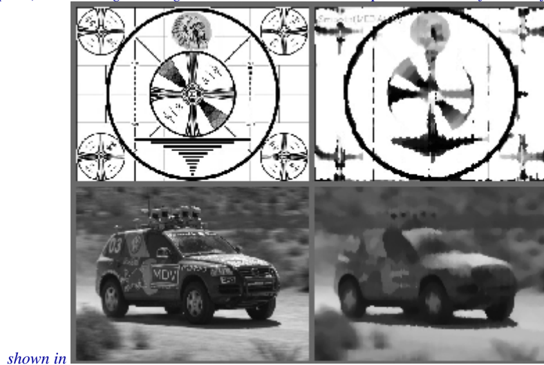
Figure 5-9. Simple blurring by averaging can be sensitive to noisy images, especially images with large isolated outlier values (sometimes called “shot noise”). Large differences in even a small number of points can cause a noticeable movement in the average value. Median filtering is able to ignore the outliers by selecting the middle points, though at a cost in speed.
